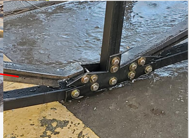
Figure 32: Failure Location - Block Shear at A2
