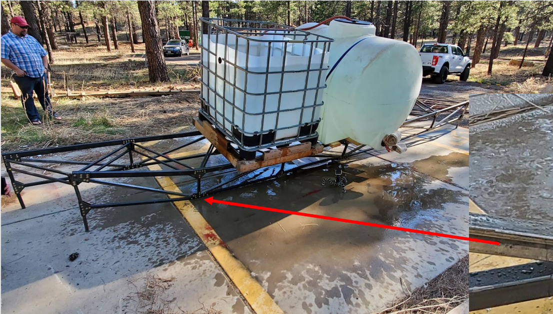
Figure 31: Bridge Loaded to Failure
